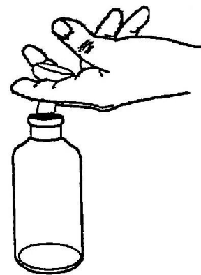
FIGURE 10. Removing a stopper from a reagent bottle
